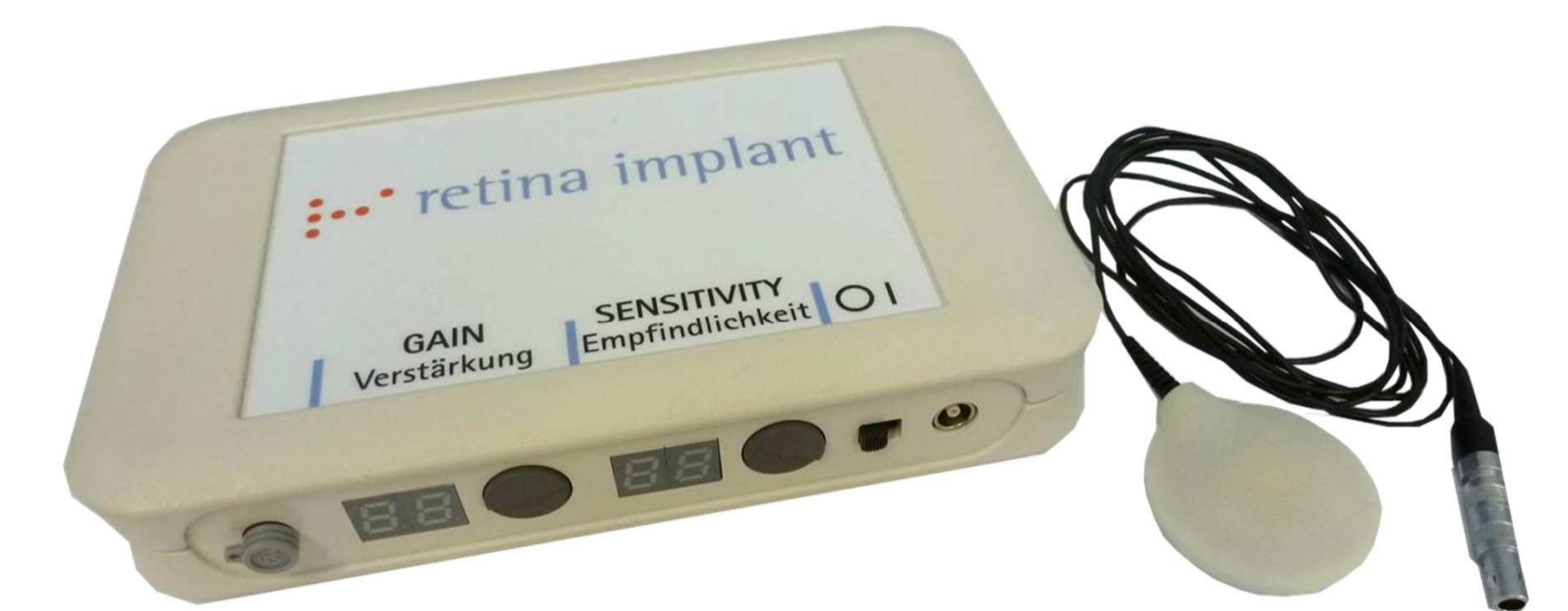
Fig. 4: External power supply with rotary knobs to adjust Gain and Sensitivity.
